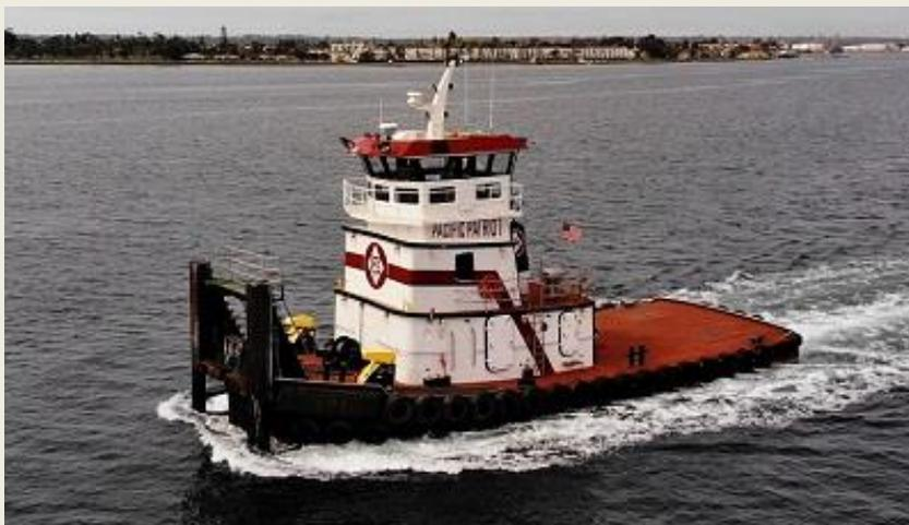
rudders are triple main and double flanking rudders. Total shaft horsepower is 1500 HP. Ship's power and hydraulics is provided by John Deere 75KW and 100KW generators. The electronics suite includes Furuno Electronics. There is berthing for four in two staterooms on the second level. A small galley, crew lounge, head with shower
